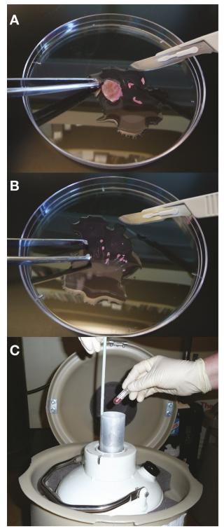
**Fig. 3. The "tissue piecing" protocol used to preserve viable cells for establishment of cell lines in the future. A)** Tissue is cut into long, thin strips. **B)** Tissue is diced into 1 mm<sup>3</sup> fragments before adding medium containing 10% DMSO as a cryoprotectant. **C)** Prepared tissue is stored in LN<sub>2</sub> until future cell culture is possible; those without cell culture capability can transport samples using a dry shipper to maintain cold-chain.
